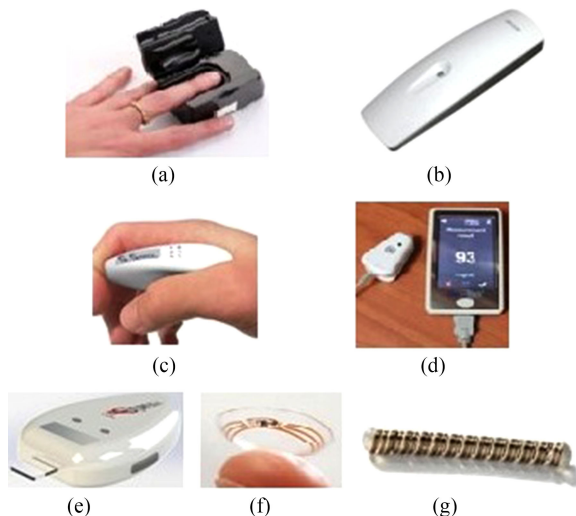
Fig. 4. Noninvasive blood glucose monitoring devices: (a) Tensor-Tip combo glucometer. (b) Glucosense. (c) GlucoWise. (d) GlucoTrack. (e) iQuickIt saliva analyzer. (f) Smart contact lens. (g) Noviosense.
