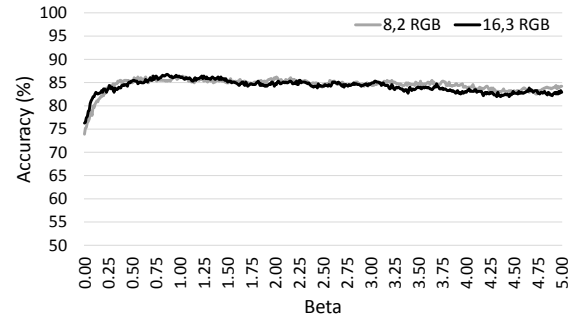
Figure 8: Accuracy obtained from the \beta parameters between (0,5] considering different configurations of neighborhoods for RGB channels.
