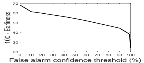
Fig. 3. Trend of Earliness with varying false alarm confidence threshold (100 - Earliness) on ASYS. Larger the value, the earlier the prediction
