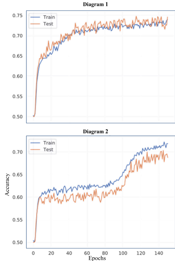
FIGURE 2. Performance of TNC embedding for f using 1 sample/min (Diagram 1) and 60 samples/min (Diagram 2).
